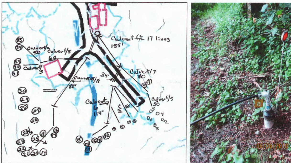
Figure 1. Dockton Springs. (Left) Map depicting the locations of the wellpoints. Pink denotes buildings; blue denotes surface water (provided by Association in 2013). (Right) Wellpoint 8. They work to keep the piping visible and out of standing water to minimize the possibility of contamination.
